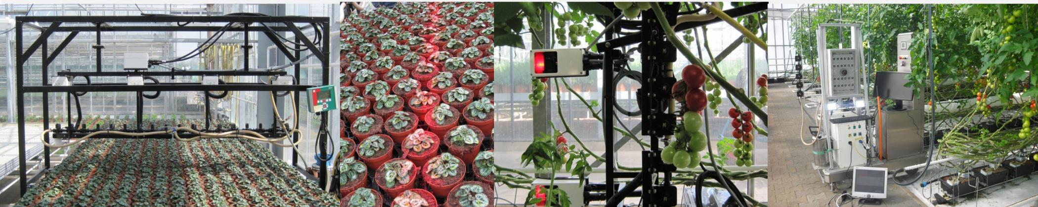
The Precision Spraying System (PSS) is a spray boom that moves through the greenhouse on a transport platform and sprays only there where needed. The PSS sprays only those areas in the crop where a sensor detected a diseased plant. The applied spray is adapted to the size and the density of the crop canopy.
